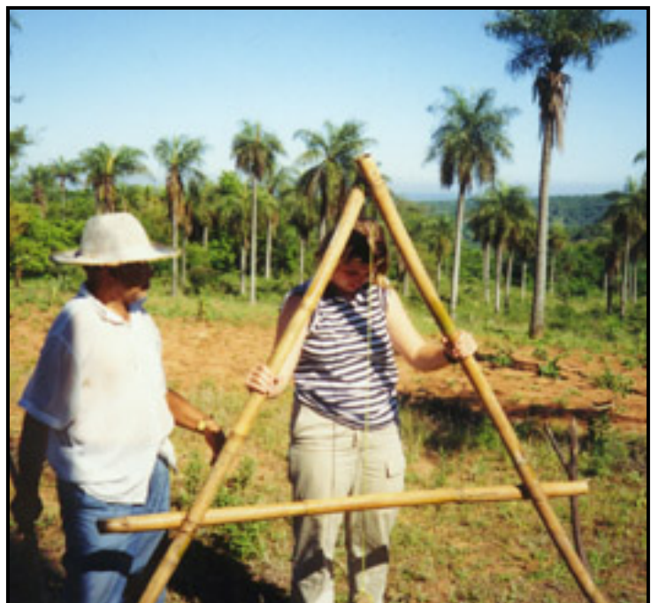
Figure App03-04: MTU Peace Corps volunteer Kristen Rahn uses an a-frame level in Paraguay in 1999.
